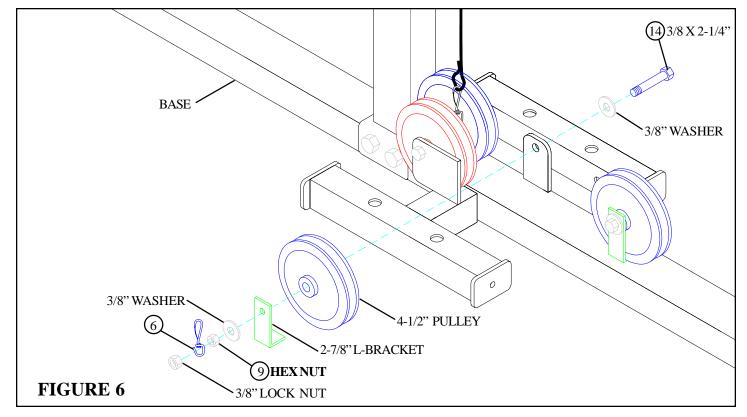
• SECURELY assemble the previously removed 4-1/2" PULLEY to the BASE using one 3/8 X 2-1/4" BOLT (14), two previously removed 3/8" WASHERS, one previously removed 2-7/8" L-BRACKET, one SWIVEL SNAP (6), one 3/8" HEX NUT (9), and one previously removed 3/8" LOCK NUT. See FIGURE 6.
